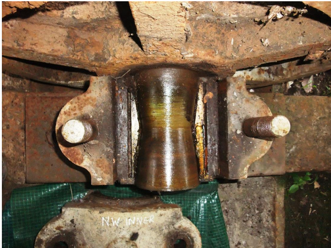
Plate 17 – NW Wheel – Inner bearing
